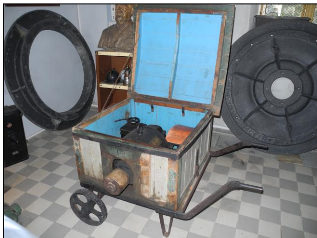
Fig. 7. Škoda handcart type VK with electric engine type SS 6 S/4 with electric performance 3.0 kW. Písek (distr. Písek). Foto J. Chmelensky, 2015.
