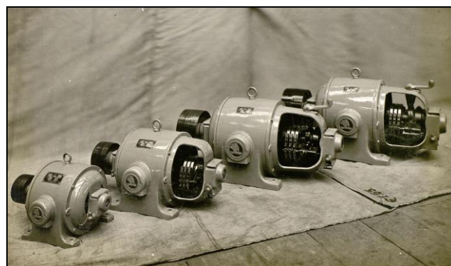
Fig. 1. The line with Škoda electric engines. From left to right: small engine with short armature, engine with armature rings and two engines with armature rings and diverters. Source: SOA Plzeň, SOA Plzeň – Klášter. Photography fund, photo n. 65-0950.
