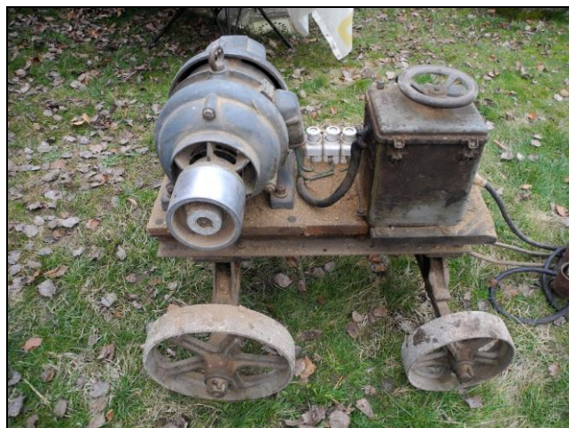
Fig. 10. Siemens–Schuckert electric engine of type DMR53N/4 wit electric preformation 5.5 kW. Own private collection. Foto J. Chmelensky, 2015.
