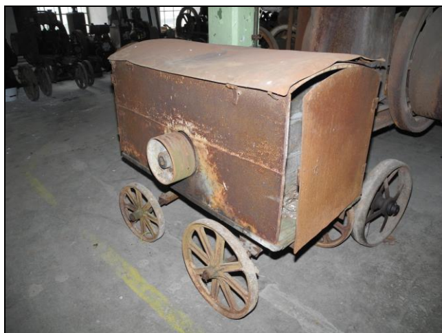
Figure 8. Bartelmus–Donát four wheel cart type VII with electric engine Škoda type AN 6 S/6-0 with electric preformation 3.3 kW. Žamberk (distr. Ústí nad Orlicí). Foto J. Chmelensky, 2015.
